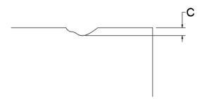
Modules that have cracks/chips which extend into areas above the copper electrodes must be rejected regardless of dimension:
