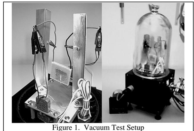
Figure 1. Vacuum Test Setup
