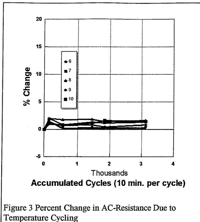
Figure 3 Percent Change in AC-Resistance Due to Temperature Cycling
