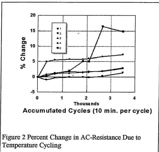
Figure 2 Percent Change in AC-Resistance Due to Temperature Cycling
