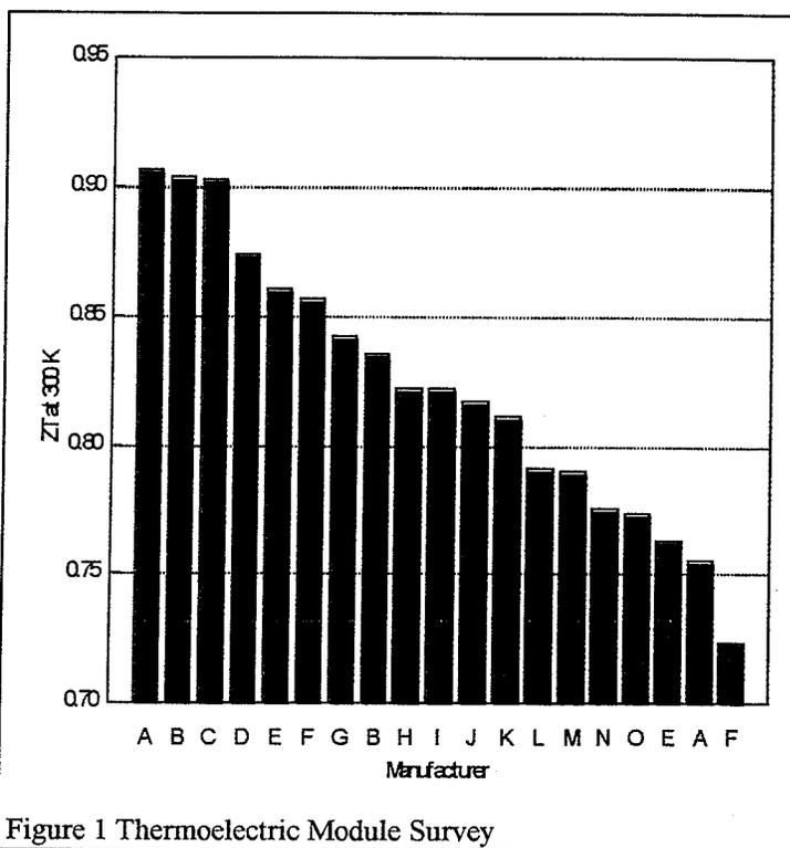
Figure 1 Thermoelectric Module Survey
