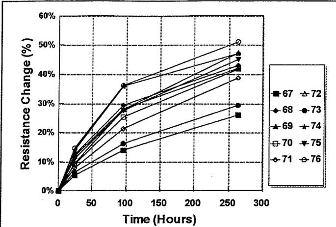
Figure 4 Effect of Exposure at 160°C on Resistance of TE Modules
