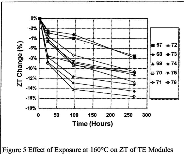
Figure 5 Effect of Exposure at 160°C on ZT of TE Modules
